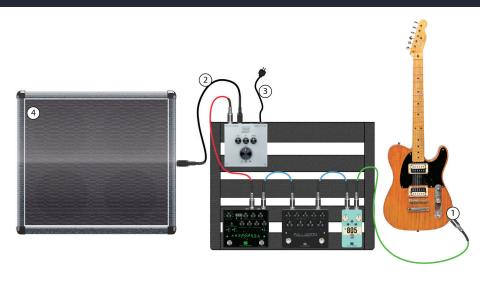
Use a high quality **speaker cable [2]** to connect your PowerStage 170's **Speaker Output jack** to the input of a **4 - 16 ohm cabinet [4]**. Using the supplied **power cable [3]**, connect the PowerStage 170 to a power outlet.
